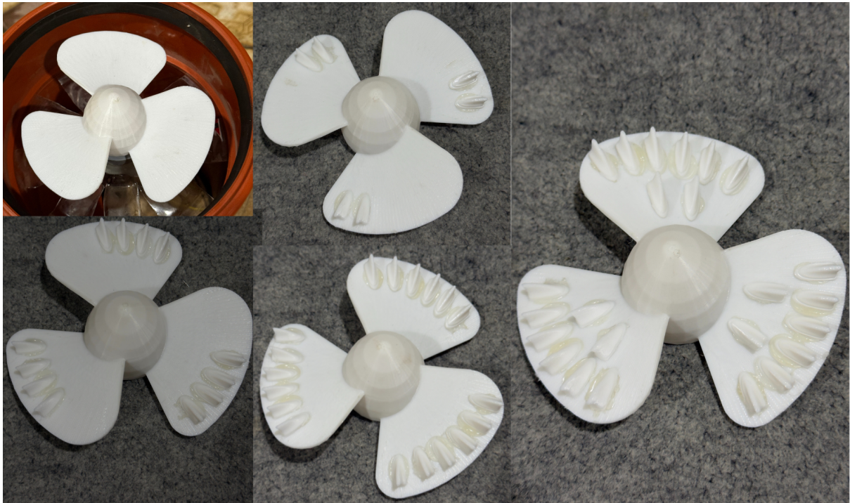
Figure 6: 3-rotor turbine design ( 0.0159 \text{ m}^2 surface area) with fins attached in different configurations (0, 6, 12, 18, 24). Demonstrating the Independent Variable
