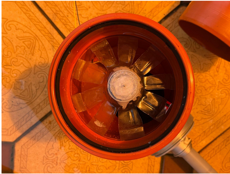
Figure 5: DC motor with waterproofing and turbine attachment, secured to minimize vibrations
