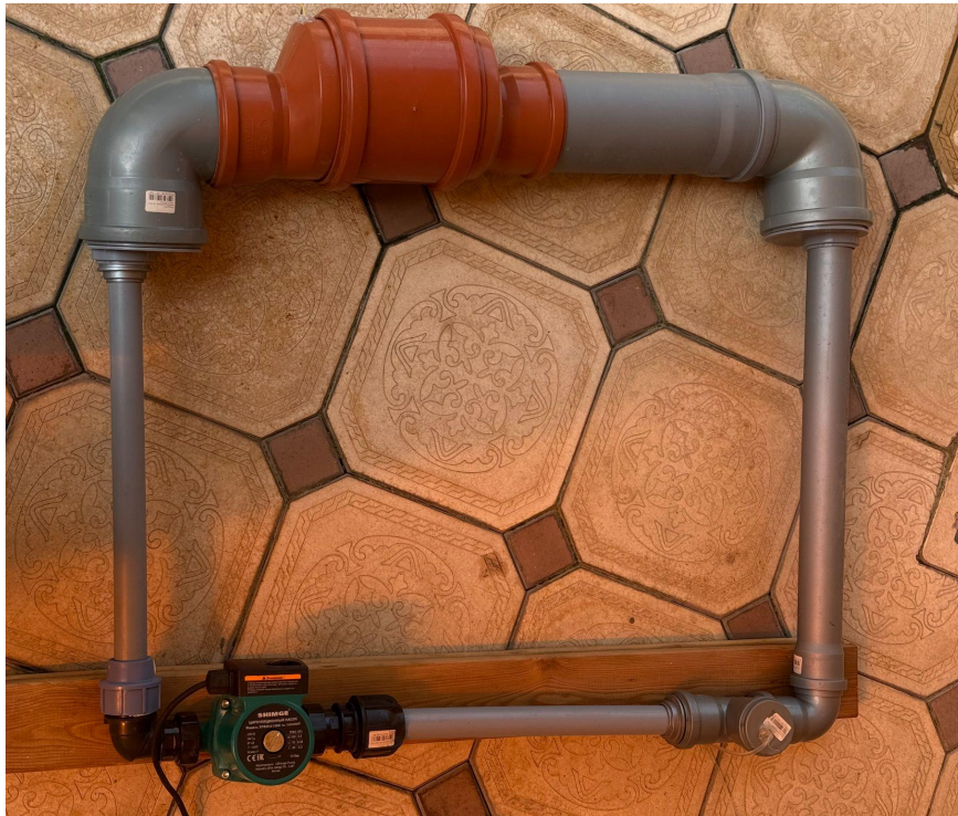
Figure 3: Complete experimental apparatus showing plumbing tube system with 150mm diameter testing section, circulation pump, and water level maintenance setup
